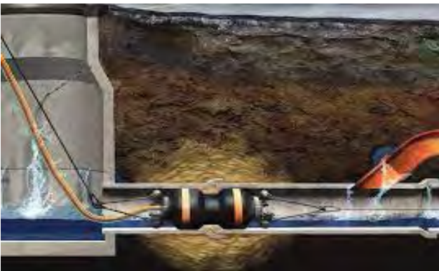
Robotic Chemical Injection grouting lateral packer pumps chemical grout into faulty joints
